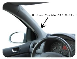
WARNING: Do Not Install Here If Antenna Will Obstruct, Block Or Interfere With Airbag Deployment
