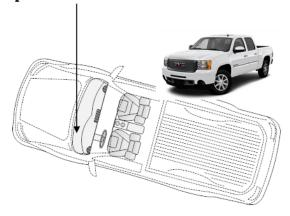
Run the cables along the side of the dash at the door hinge, and place the transceiver box under your dash. For best results, consider using a zip-tie to secure the transceiver to ensure it doesn't fall from beneath the dash.
