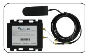
Place the antenna (with the embossed letters "GPS" facing UP) on your dash at the base of the windshield.
