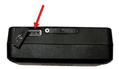
To Charge The PT-8100 Insert The USB Cable Into The USB port on the PT-8100. Charging Time Is Approximately 6 Hours. Once Fully Charged Expect 8-10 Motion Hours Of Live 10-Second GPS Tracking. When the device is not moving, it enters standby mode to save battery power, it updates positions every 8 hours when not moving.
